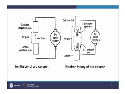
So, what happens that the creation of the arc, there are two theories for the creation of this arc. Now, there is iron theory of the arc column, now the thing is, that you have a positive electrode you have a negative electrode. So, once you have arc connecting that to a power supply, now what happens? That the ion theory of the arc column tells that you will have the flow of iron from the anode and it will move towards the cathode. So, that is the theory of the iron theory of the arc column.
