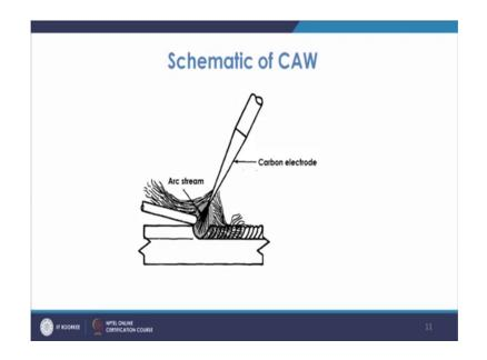
The arc stream is generated you have, and the weld bead appears like this. So, this is the one of the variety of the arc welding, we will discuss more about on the principle of generation of arc and also about the different processes in the coming lectures.
