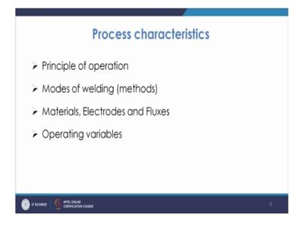
As we talk about the operating variables; now, operating variables are normally here the a welding current which is normally quite larger value is taken depending upon the degree of penetration which can be used. You have voltage also voltage basically, you know, if you take a larger voltage it will talk about the, you know, flame dispersal so, it will go and heat in the larger portions.
