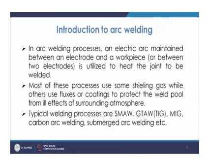
So, basically in that case you have a flux which is there and then that flux in. So, normally the electrode is coated with flux, and this is normally a you know electrode which is normally consumable, and then once it consumes it has coated with flux, this flux melts and creates one environment around the weld pool.
