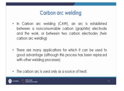
Then, the next type of a welding is also one is carbon arc welding. Now in the carbon arc welding the arc is between the non-consumable type of carbon or graphite electrodes, which are used for heating the work. And then this way either you have the twin carbon arc welding also. So, now there are many applications which can be, you know, it has many advantages.
