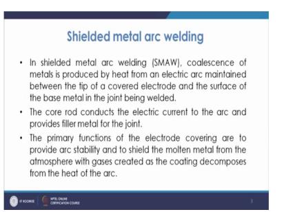
Now, here the rod which is there, that basically melts and that will basically conduct the electric current, and it will conduct the electric current to the arc, and it will also provide or it will work as a filler material for the joint. So, what happens that, the electrode which is connected a electro holder, now it has since it is a metal it is carrying the current, and producing the arc and getting consumed so, that way you are using that electrode also as the filler material in that case.
