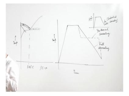
So, what we have this is are the iron carbon diagram so, here this is the you know, this is the lower critical temperature of 723 degree centigrade and this is your upper critical temperature that is a three line. So, this is your A 1 line and this is your A 3 line now
