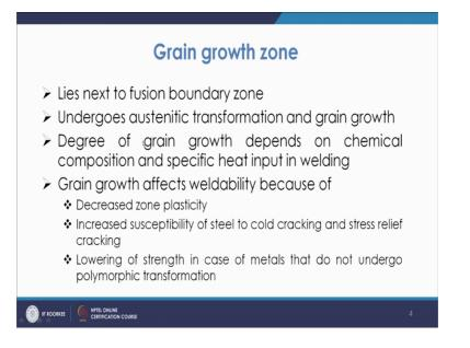
Now, it goes undergoes the austenitic transformation and grain growth so, as the temperature goes (Refer Time: 22:27) acceleration started at certain temperature and then once you go to the larger temperature zone, you will have grain growth started. So, that
