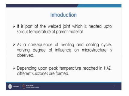
So, as we know that once you have a zone then after the weld metal zone the zone starts which is partly melted, then after that the zone is the grain growth zone under beat zone is there then you have the adjacent to its the grain growth zone. So, it has upper and lower boundaries then after that you have the, you know grain refinement zone further you have partly transformed zone and so.
