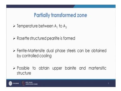
Now, next will be your partially transforms zone, now in the partially transformed zone that temperature is normally between 750 to 950 degree centigrade so, normally it is between the lower critical to upper critical temperature. So, if you look at this figure it is through this is a lower critical temperature and this is the upper critical temperature in between you see that this is the partially transformed zone which is observed.
