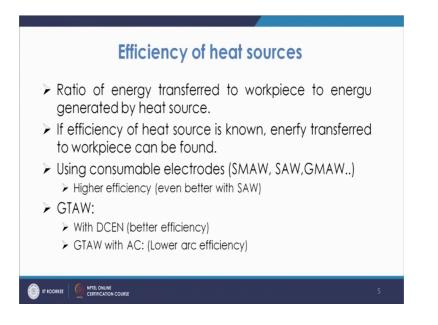
Now coming to the efficiency of heat sources, what is the efficiency of heat source now it is that we use the heat source to basically transfer the energy to the work piece. So, you have certain energy which is of the heat source, and how much energy has been used by the having transferred to the work piece. So, that energy which is transferred to the work piece, at that divided by energy generated by the heat source that basically is known as the efficiency of each source.
