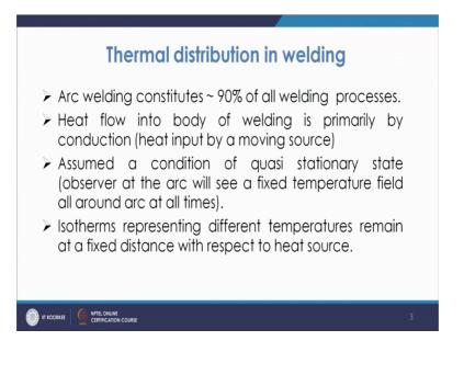
So, what we see that most of the welding processes are. So, about 90 percent of the welding process which we talked about, about 90 percent is based on the arc welding process. So, among the in the all the fusion welding processes, you have about 90 percent is you know from the arc welding because arc welding is simple and it is very effective. So, normally we use the arc welding process.
