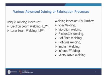
Now, these are basically we have to join to various thin point. Now, if that is not possible by normal welding process so that can be done by electron beam welding, laser beam welding or maybe sometimes for extremely hard materials or extremely high melting point materials. So, on those cases where about the conventional welding operation is not power you know suitable we go for such kind of unique welding processes.
