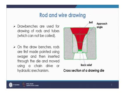
So, using that chain drive or hydraulic mechanism you can do this pulling operation. So, you have basically there is dye and then you will have the dye holder. So, basically normally this dye is host in some you know case. So, that is becoming, this is your dye and this is becoming the dye holder. So, that is how you have the dye holder and then with the jaw you grip this whole rod and then you further you know pull it. So, that is how you try to do these drawing operations.
