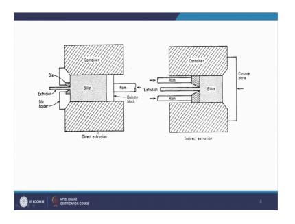
So, you have the, this is the case of directors extrusion. So, the billet is placed in the container. So, this is the container and you have the billet placed here, and then this is a ram. So, the ram is here and you have a dummy block or you also call it as the pressure plate.
