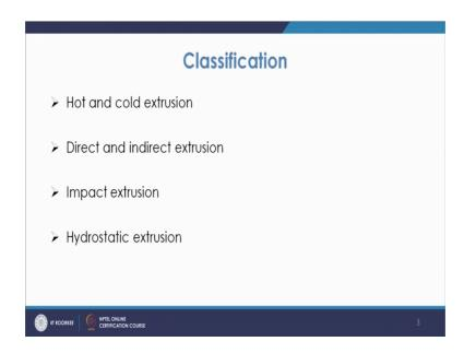
So, in the hydrostatic extrusion what we do is, that the pressure basically is applied the hydrostatic component of stress is used to apply the pressure. So, this way the lubrication which is there the lubrication is better in that sense and. In fact, this says that even and the brittle materials also are extruded in that case because you apply the hydrostatic pressure, and then that because of that pressure of the metal is confined to go through the opening.
