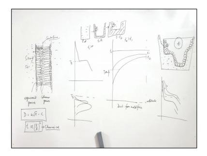
So, as we see that once you have the liquid in this liquid touching this boundary and here everywhere is liquid basically; all is liquid. So, once it touches this boundary and in that case if it is there, is a heterogeneous nucleation condition and it is practically that, whenever we cast any material. So, in that case if this is the mold wall, it is at lower temperature and it has many sites, where the nucleation starts.
