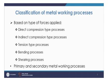
So, if you have the direct compression type forces means, the compressive stress compressive force is directly applied to the surface of the body, and in that basically the metal will flow at right angles to the direction of compression.
