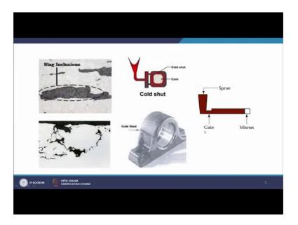
You have the slag inclusions which you see slags are they are inside this structure. So, this is the example certain slag inclusion you see the cold shut here and misruns.
