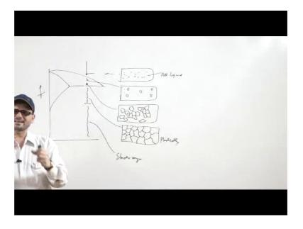
What you see that. So, what happens, that in case of the alloys as the temperature will come down. So, this is temperature, as the temperature will come down at this point you have completely liquid, this structure is completely liquid all liquid. Now once it comes here in this one then in this zone basically you have a small amount of solid crystallised
