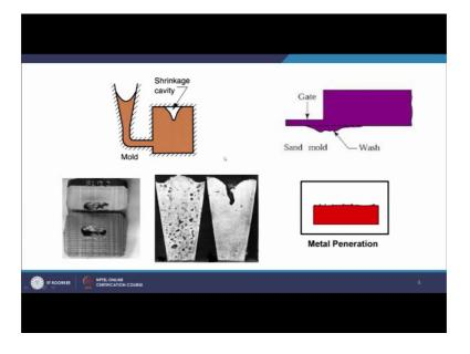
You go to the cavity you have shrinkage cavity as you see this is a casting where you have got in the last portion which is the solidified you have the cavity appearing in this fashion which looks into the structure like this, also you that see that the shrinkages at different places in that here and you see that this kind of piping is there available in the this is because of the shrinkage. So, these are the shrinkage examples wash in this figure
