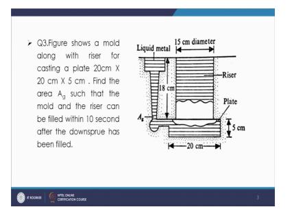
Next question is that in the figure it is shown that you have a riser, I mean along the riser it is shown. So, there is a one riser which is also to be filled. So, as you see that you have the liquid metal it is going through the down sprue and in the bottom it has. So, using the top gating it is filling the mold cavity, and using the bottom gating basically again it is filling the riser.
