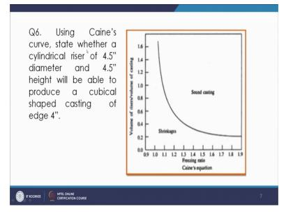
You can see another problem of another just a problem where this it is written that using Caines curve whether you can say that it is an integral riser of 4.5 inch diameter and 4.5 inch height will be able to produce a cubical shape casting of edge 4 inch.
