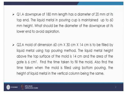
So, you have the dance blue and also the liquid metal in the pouring cap is maintained up to 60 mm height. So, the first problem is that you have a pouring cup and you have a down sprue and this is the pouring cup height and this pouring cup height is a maintained as 60 mm and the down sprue is of length 180 mm.
