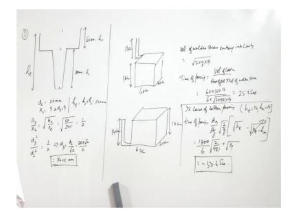
So, this length is 180 mm. So, then what should be the diameter of the down sprue at its lower end to avoid aspiration. So, basically as you know that we define 0.1, 0.2 and 0.3. So, this height is h 2 and this is known as h c this is 60 mm and. So, what we see is that r is A 3 by A 2 that is basically under root sc by ht. So, ht is this total height, and you have to find the. So, this value is given the diameter of 20 mm top ends.
