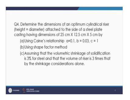
So, let us say by different methods we will try to solve such problems. Now, here the question is given as that you have to determine the dimension of an optimum cylindrical riser, attached to the side of a steel plate having casting plate casting having dimension of 25 by 25.5 by 5 centimeter using Caines relationship. So, as you know that a b and c value is given and you have to find the value of the diameter of the riser using the Caines method.
