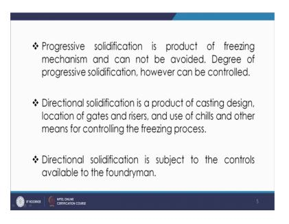
Now, in the case of the progressive solidification as it is written that is the product of freezing mechanism and it cannot be controlled avoided. Although you can control its degree it has to start, if it is touching the walls of the surface where the under cooling is more the temperature differential is there wherever the temperature will be less from there the nucleation will start if that favoring condition is achieved. Like the temperature
