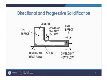
Now, if you see this geometry this figure what you see is when you are casting the liquid metal into the cavity then what you see is the immediately the solidification front will start moving inward. So, from this side it will moved in this direction from this side it will move in this direction from this side it will move in this direction this way and this way or so.
