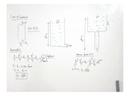
So, in that if the rho is basically rho is the density of fluid, A is the area of cross section of the channel and V 1, V is the velocity. So, if you have two points, so if you have two points then at one and two, so if the area is same if it is area is A 2 and this area is A 1 then A 1 V 1. So, this is V 1 and this is V 2. So, A 1 V 1 will be A 2 V 2. So, this is for
