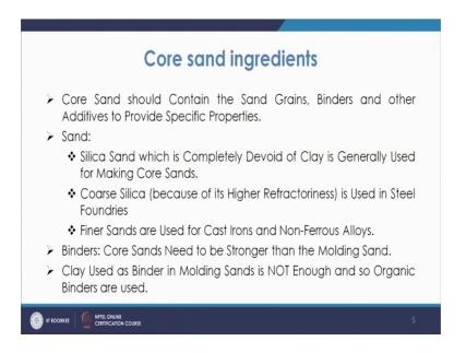
Next we will discuss about the core sand ingredients. So, as you see the core sand they contain the sand grains, binders and other additives to provide the specific properties.
