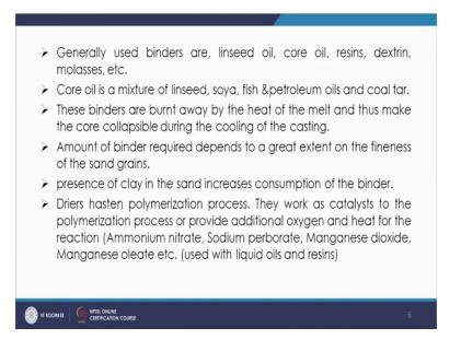
Also in that now core oil is a mixture of linseed soya, fish and petroleum oils and coal tar. So, that is core oil and these binders basically what happens they are burnt away by the heat of the melt and then once they burn then basically they provide the space and in that case they make the core collapsible during the cooling of the casting.
