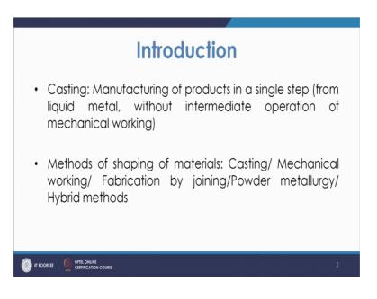
So, coming to the definition of casting, basically casting is defined as the manufacturing of products in a single step from liquid metal, without intermediate operation of mechanical working.
