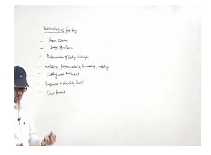
So, if you talk about typical forming processes, so in the technology of founding or technology of casting, what you see is, initially you have basically some design in mind. So, you have the process selection, design specification, you have determination of casting technique, further you have molding pattern making, core making. Then once you have also the melting units, 1 after that you have see product ready then you go for fettling and heat treatment, inspection and quality control.
