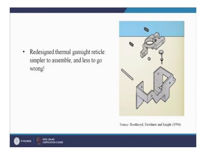
And this is a redesign it is going the redesigned part or the product is going to achieve the desired function as was being done by the previous design, but here you see, far less number of fasteners and the parts have been redesigned in such a way that they are easy to assemble. Now what are the advantages or improvements noted, assembly time improvement is 84 percent, number of different parts original design had 24 parts.
