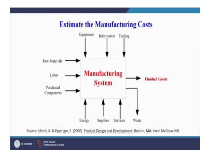
What are the various inputs; raw materials, labour, purchased components, for sub assemblies, equipment, information, tooling, energy, supplies, services and then sometimes we have some rejected parts that go as waste. So, our final product are the finished goods only. So, we have to focus on each and every element, each and every component of this system in order to overall optimise the manufacturing process
