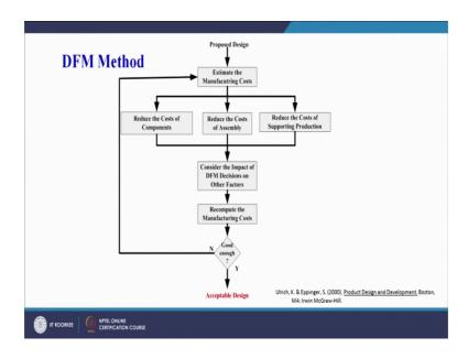
There is a proposed design which already has taken into account the concepts of value engineering, it is satisfying all the functions as specified by the customer. So, we have a input that is a product design or a concept design. We will see, as per DFM, what are the manufacturing cost. So, in the previous slide we have seen that the manufacturing system is made up of so many inputs.
