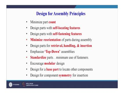
I have already highlighted some of them. Minimise the part count; number of parts should be less. Design parts with self-locating features; so, part should be so designed that they locate a one above the other easily.
