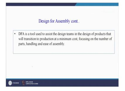
Now, DFA is a tool used to assist the design teams in the design of products that will transition to production at a minimum cost focusing on the number of parts handling and ease of assembly.
