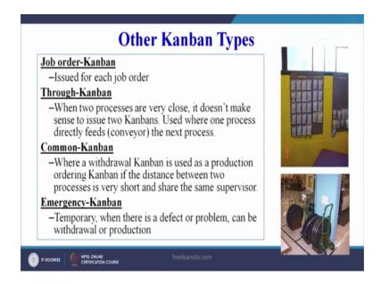
Now there can be other types of Kanban which can be job order Kanban issued for each job order. Through Kanban when two processes are very close it does not make sense to issue two Kanbans used where one process directly feeds the next process. So, maybe if on a conveyor belt type of Kanban conveyor belt type of material handling system or the process line, we can use a through kanban. So, if there are two processes happening need not issue two Kanbans.
