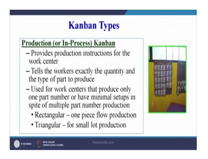
Now, Kanban types we can see with the figure also here. Production or in process Kanban provides production instructions for the work center. As I have already discussed that if there are three workstations from third workstation, we will send a signal to the second workstation regarding the requirement. So, provides production instructions for the work centers tells the workers exactly the quantity and that and the type of the part to produce.
