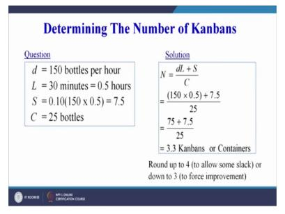
So, we can see the question here determining the number of Kanbans, you can see the question d is the demand rate which is which was I have already told numbers with respect to time. So, 150 bottles per hour is the demand rate. L is 30 minutes that is 0.5
