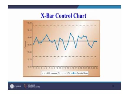
This is a black line represents the center line which was fifteen point you can see 15.92. So, this is corresponding to 15.92 value and then these are the value sample mean how the sample means are changing so, so, many samples we have taken.
