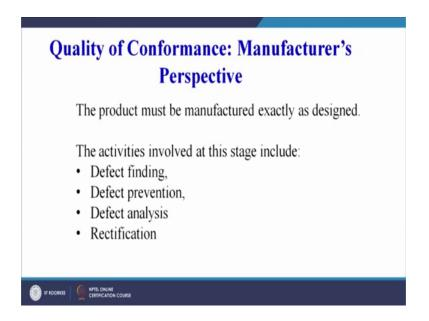
The activities involved at this stage may include defect finding, defect prevention, defect analysis, rectification which means that we have to conform to the specifications as designed. So, whenever a designer designs a product he lays out certain specifications for the manufacturer.
