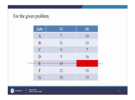
So, here we can see we have now done the summation of first and second column for machine G and second and third column for machine H and we get these values. Now this is a simple problem here we can see we have 7 jobs processing times on a machine G and processing times for machine H.
