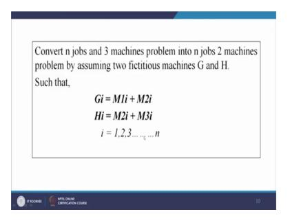
So, convert n jobs and 3 machines problem into n jobs and 2 machines problem by assuming 2 fictitious machines G and H. Now for G for first job what is the time processing time, processing time is the processing time required on machine 1 and processing time required on machine 2.
