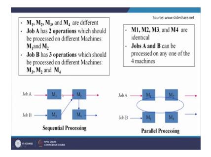
These are four machines M 1, M 2, M 3 and M 4 and all four machines are of different types. This is an example of sequential processing M 1, M 2, M 3, M 4 are different job A has two operations which should be processed on different machines M 1 and M 2. So, job A goes to M 1 and M 2 and finally, goes to the next level.
