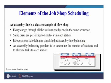
Shop where maybe; we are starting our assembly from one end of our assembly line, that the final product comes out from the other end of the assembly line. So, an assembly line is a classic example of a flow shop. So, we can see every car go through all the stations one by one in the same sequence.
