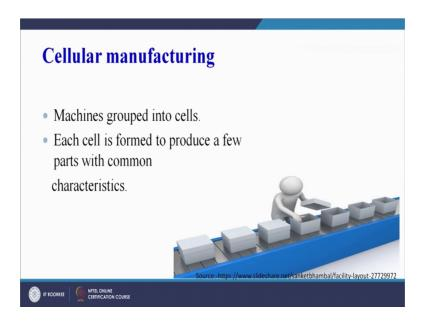
Now, in cellular type of layout, we have machines which are grouped into cells. So, we will try to understand this with the help of a diagram and each cell is formed to produce a few parts with common characteristics. Before explaining the concept of cellular manufacturing, I would like to invoke another word that is group technology; because here we are producing few parts with common characteristics.
