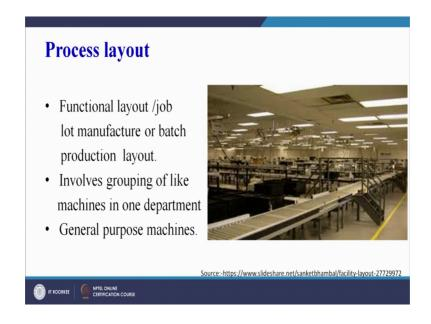
So, let us start our discussion with the Process type of layout. Before we understand the process type of layout, I must question that what are the limitations of a product type of layout or a line type of layout? The advantages all of us know; because there is a particular sequence or not much planning is required.
