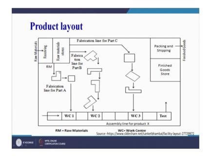
Now, this is an example of a product type of layout, you can see. The raw materials this is a raw materials being received here; raw materials store. So, Fabrication of part A, it is coming to WC 1 and then, this is Fabrication of part B, again WC 2; Fabrication of part C coming here and all these 3 assembly line of the product which is coming here and finally, after testing it is going to packaging and shipping and finished goods store.
