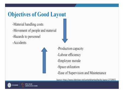
You can see 2 arrows here. Now the top arrow is pointing downwards which means that these 4 factors we need to reduce, when we are designing a layout or a good layout should focus on minimizing these 4 factors that are given here.
