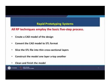
Now, all RP techniques employ the 5 step process. So, basically there are 5 steps or 5 stages in which we can make a prototype. So, first of all what we have to do? We have to create a CAD model of the design. So, CAD is computer aided design. So, we have to use any software and make a 3-D model of the design.
