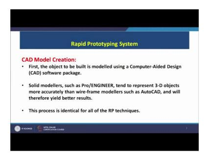
Now, CAD model creation first the object to be built is modelled using computer aided design I have highlighted already. Solid modular such as pro engineer tend to represent 3-D objects more accurately then wireframe modular such as auto CAD and will therefore, yield better results. Now, that is from the CAD point of view that once you are making a CAD model of your product you need to make a judicious decision that which
