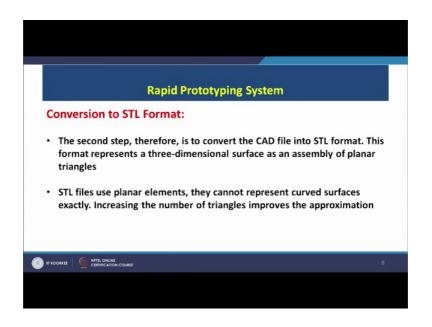
Conversion to STL format, but maybe the previous was that the CAD model is required for almost all rapid prototyping technologies. Conversion to a STL format the second step therefore, is to convert a CAD file into that steel format this format represents a three dimensional surface as an assembly of planar triangles. So, we have to convert it into this format that CAD file into STL format.
