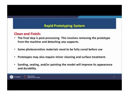
Clean and finish, the final step is post processing this involves removing the prototype from the machine and detaching any supporting structures. Some photosensitive materials need to be fully cured before they are used. So, we have to use additional maybe heating mechanism or additional furnaces to fully cure these resins before making them fully functional prototypes.
