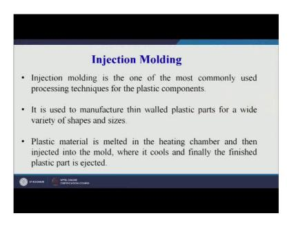
Now, injection molding is one of the most commonly I have told this is a commercial process industrial scale process used for plastic components. So, it is not something which we can say is in the research stage, already different companies are making different types of injection molding machines. And at IIT Roorkee we have a injection molding machine which we are using for conducting our research work. So, it is a
