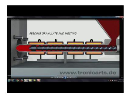
Now, the screws rotating and the material is moving down the cause of these heating elements it will get melted and this is a nozzle. So, here with this is the mold.
