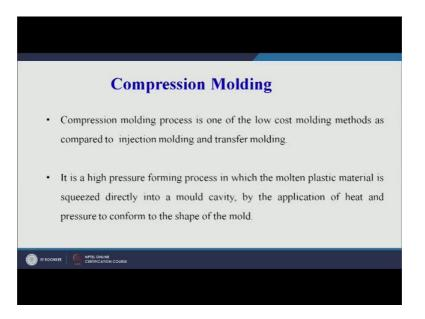
Compression molding process is one of the low cost molding process, why is it is low cost? Because of the set ups that we use, because of the control parameters that are there in compression molding; they are easy to control and this low cost we are comparing it; with injection molding and transfer molding. So, maybe injection molding we have not covered till now, but maybe in the subsequent sessions. We will talk about injection molding of plastics also.
