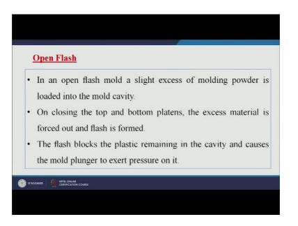
First type is the open flash type; in open flash mold, a slightly excess of molding material is loaded into the mold cavity. First point we should keep in mind; that as per the amount of charge required inside the mold cavity, we will keep slightly additional material inside the mold cavity. On closing the top and the bottom platens; that is the top and the bottom halves of the mold; the excess material is forced out and a flash is formed.
