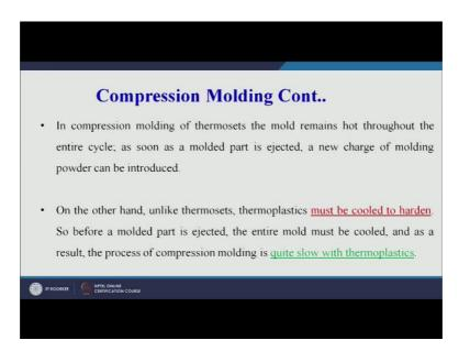
As soon as a molded part is ejected, a new charge of molding powder can be introduced.
