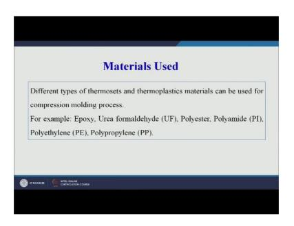
So different types of thermosets and thermoplastics can be used in compression molding process; for example, Epoxy; very common type of thermoset material, Urea formaldehyde, Polyester, Polyamide, Polyethylene, Polypropylene; all these raw materials can be used. So, Polyethylene, Polypropylene both are thermoplastics category and Epoxy, Polyester are in the thermoset category.
