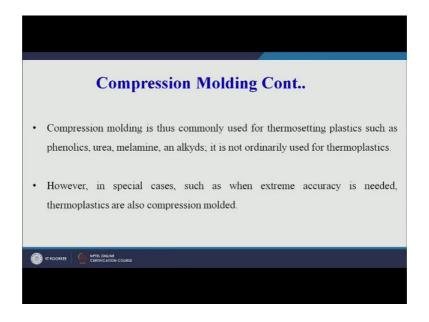
Compression molding is thus commonly used for thermosetting plastics; such as now what are the materials that are commonly used for compression molding process? That
