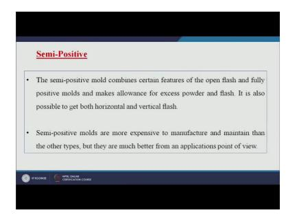
So, we will not exactly put the metered amount; slightly excessive raw material we will input inside the mold cavity. So, it will form slight amount of; or may be smaller flash as compared to a open flash type. And it is also possible to get horizontal and vertical flash; in case of semi positive type of mold.
