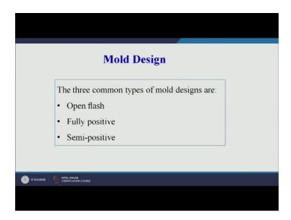
We can see the three common types of mold designs are; open flash, fully positive and semi positive. So, we will see each one of these and then we will try to see the diagram and try to understand that what are the advantages as well as limitations of the three important types of designs that are mold designs used for compression molding process.
