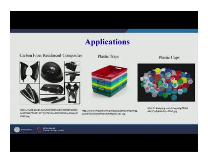
Plastic trays; all of us use these trays, when you travel by air; during the security check; these type of trays are there. So, you can make different types of plastic caps also using compression molding process; then even helmets these are the carbon fiber reinforced composites; right now our session is on compression molding of plastics.
