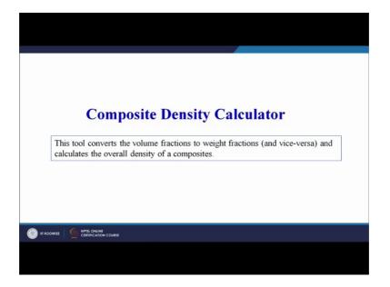
Then in the same website there is a composite density calculator. So, this tool converts the volume fractions to weight fractions and vice versa and calculates the overall density of the composites. Here also we have to input the information inform of the fibre the resin and finally, the system will calculate the density of the composite develop based on the fibre and the resin.
