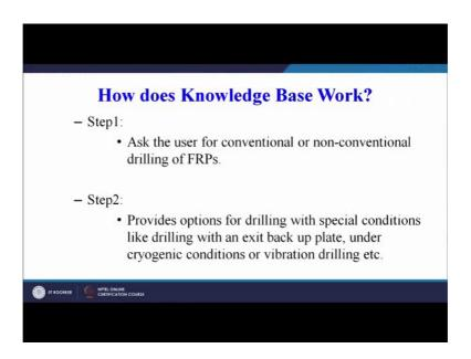
In step 1 the system will prompt the user or it will ask the user for conventional or nonconventional drilling of fiber reinforced plastics.
