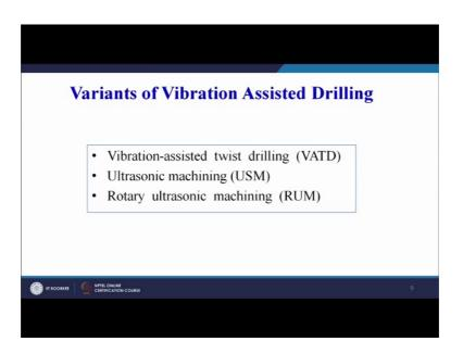
Now, different variations or variants of vibration assisted drilling are investigated in research. Vibration assisted twist drilling, where the drill that is used is a twist drill, standard twist drill, ultrasonic machining, then rotary ultrasonic machining. So, whatever we have seen it is ultrasonic assisted drilling UAD, we can have the same variant is the vibration assisted twist drilling.
