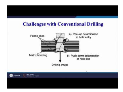
So, this is one form of damage we can see here on your screen; this is a push down type of delamination, this is because of the thrust force generated during the contact of the drill with the laminate. Then there is a peel up delamination these fibers; these fibers represent the peel up delamination, this is the pushdown type of delamination towards the exit of the drill; then there is matrix de bonding also, sometimes the matrix may fail.
