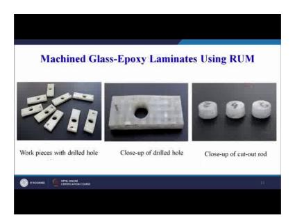
So, this is the result; we can see this is a glass fiber reinforced epoxy composite, these are the hole successfully made without much damage; workpecies with the drilled hole. So, so many work pieces have been drilled using the rotary ultrasonic machining technique. And this is a close up of the cut out rod; so, if you use a hollow tool; it will
