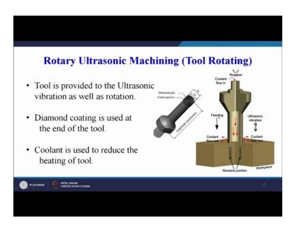
This is rotary ultrasonic machining, the tool is rotating; tool is provided the ultrasonic vibration as well as rotation; as I have already highlighted. Diamond coating is used at the end of the tool, coolant is used to reduce the heating of the tool.
