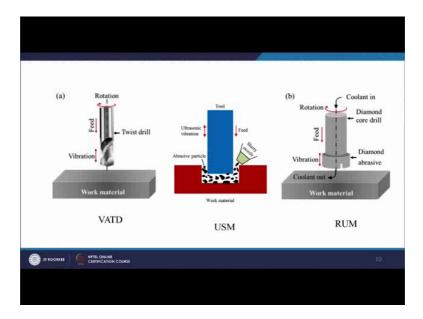
So, this is our vibration assisted twist drilling with the help of diagram, we have tried to explain. The first one is the vibration assisted twist drilling; VATD; vibration assisted,
