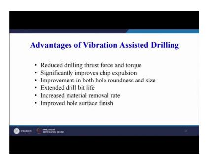
So, what are the advantages? The advantages are reduced drilling thrust force and torque which we have already seen with the reference of one of the research articles.
