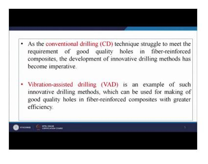
As the conventional drilling technique struggle to meet the requirement of good quality holes; so, we have seen that there are different forms of damage that takes place and conventional drilling leads to this form of damage in fiber reinforced composites. There is a eminent need to develop innovative drilling method, that can reduce this effect of damage.
