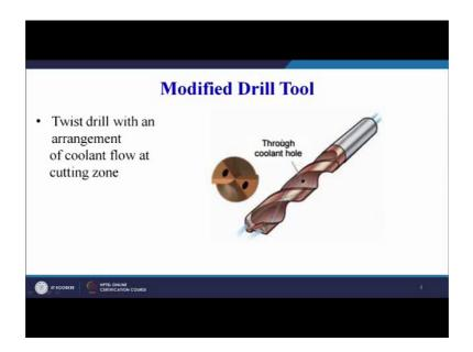
Then we can see the modified drill point geometry this is further modification here you can see there is a through coolant hole here these are the two holes. So, the twist drill with an arrangement of coolant flow at the cutting zone. So, different types of tools geometries can be investigated for optimizing the drilling performance of the polymer composites and this can be one drill.
