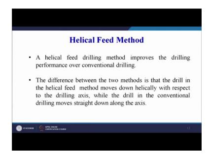
So, you can see a helical feed in helical feed drilling method it improves the drilling performance over the conventional drilling how it improves, what is the difference that has been clearly outlined in second point.
