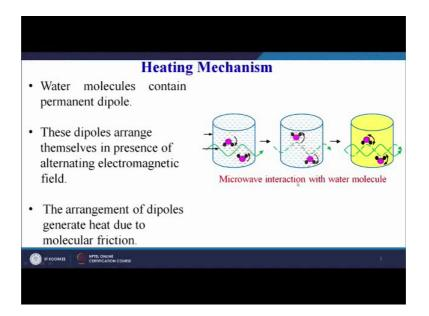
And this is the example of a water; so, water molecules contain a permanent dipole. These dipoles arrange themselves in presence of the alternative electromagnetic or alternating electromagnetic field. The arrangement of dipoles generate heat; due to molecular friction.
