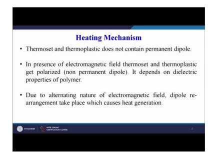
Now, thermoset and thermoplastic does not contain a permanent dipole; that is may be one challenge; so, they do not have a permanent dipole. But in the presence of electromagnetic field, thermoset and thermoplastics get polarized; they are means although they do not contain permanent dipoles, but yes non-permanent or semi permanent dipoles can be there or they can be generated on exposure of the electromagnetic fields.
