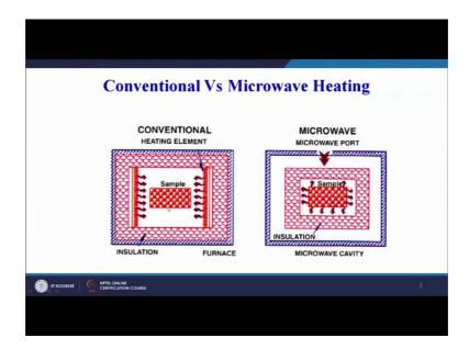
And this is our sample that we want to heat. So, our heating element will first become hot and then it will try to heat the sample by supplying heat to the sample, which is kept inside the furnace.
