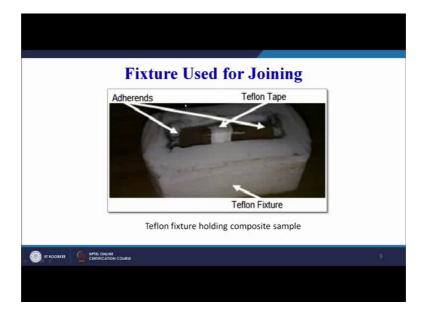
Now, this is a fixture that is used for joining; these are our own experimental findings. So, this is a adherent number 1 on your screen, this is adherent number 2 and this white color teflon tape is used to join the 2 parts or to bind the 2 parts together or to keep the 2 parts intact or 2 adherents intact at the joint overlap area. And this is a fixture which is used, now what is ideally required is that these 2 parts must join successfully.
