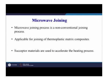
So, let us now start our discussion; you can have on your screen; microwave joining process is a non conventional joining process. I have already highlighted, emphasized outlined in the very beginning in today's session that adhesive joining and mechanical fastening are the 2 most important joining techniques which are used for joining of polymer based composites. But microwaves can also be used and it is an unconventional way of joining the 2 composite parts together.
