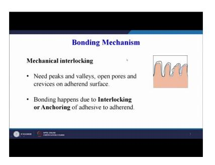
Now, this is the bonding mechanism which usually takes place between the 2 mating parts or 2 parts to be joined together. First bonding mechanism is the mechanical interlocking. Must I tell you that these types of peaks and valleys will not be available on any surface? Surfaces are usually very smooth specially in case of polymers and polymer products.
