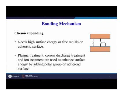
So, first requirement for chemical bonding is that you need to have high surface energy or free radicals on the adherent surface.
