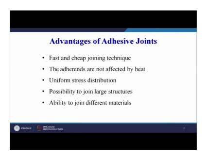
So, we will see quickly that what are the advantages. They are fast and cheap. Joining technique, the adherents are not affected by heat because we are only applying the adhesive and then, we are joining them together.
