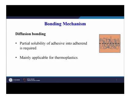
So, this top one is our first adherent, this can be the second adherent at the joint interface, the entangling of the polymer chains or diffusion of the polymer chains at the interface will add to the bonding of the 2 adherents. So, partial solubility of the aggressive into the adherent is required.
