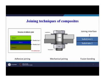
So, we can see here we are calling it as a adherent. This is adherent or substrate 1. You can call it a substrate also. So, substrate or adherent 1, this is substrate or adherent 2 and this is the adhesive, blue colour adhesive applied between the two. Now, this is just to explain that how joining can be done using an adhesive.
