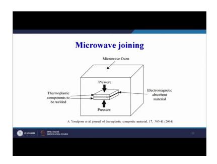
These are the 2 we can say adherent thermoplastic components. Well, this is our first component. Second component in between we have put this black solid line depicts the electromagnetic absorbent material which will absorb the electromagnetic waves or the microwaves and when pressure will be applied because of the heating effect induced by the electromagnetic absorbent material, there will be adjoint that will be developed between the 2 thermoplastic composite materials.
