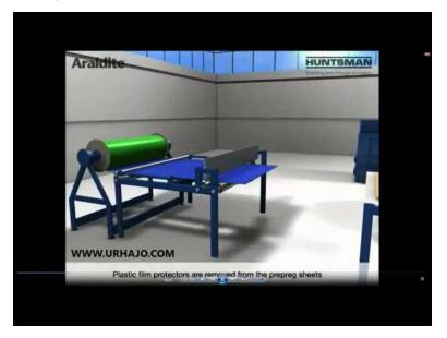
This is basically the prepreg; that is coming. This is the role of the prepreg, and the prepreg is moving in this direction, and here we have a cutter which will cut the size as per the required dimensions. Now let us start it. So this prepreg, two sheets are being removed from there, at this prepreg is finally a stacked prepregs are going inside the mold, the next prepreg will come and it will again fit inside the mold, as per the required design of the mold.
