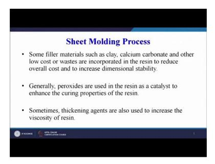
So, some filler materials; such as clay calcium carbonate and other low cost or wastes are incorporate in the resin, to reduce the overall cost and increase the dimensional stability.
