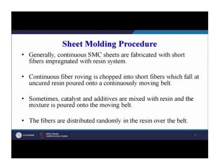
So, maybe continuous SMC sheets are fabricated with short fibers impregnated with resin system. So, here we will not have long fibers or woven mat form of fiber. We will have shot chopped fibers, which will be used as the reinforcing agents for the thermosetting type of polymers.
