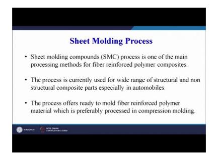
So, sheet molding compounds is one of the main processing methods for fiber reinforced polymer composites. So, it is half cooked, half-baked material which is fully cured to make a composite product.
