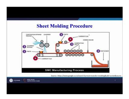
So, you can see sheet molding procedure. Let us first see this is a moving belt, which I was talking about. This is a moving belt continuously rotating. This is a red color is the carrier film, on which our both the constituents; the resin and the short fibers will fall.
