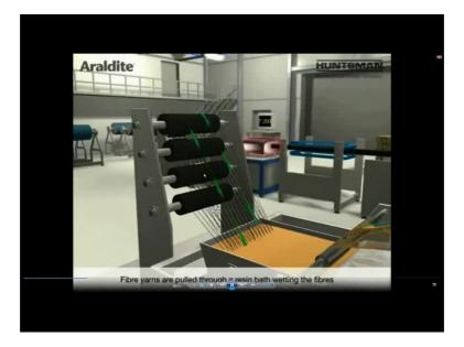
We can see here, this is the pultrusion setup. It is it is a large sized set up. So, here we see these are the rovings. Fibre yarns are pulled through a resin bath, wetting the fibres. This is a resin bath. Fibres are coming from here and getting wet in the resin impregnation system.
