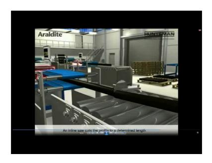
And this is the cutting mechanism, where the saw cuts the profiled it or determined length, predetermined length.
