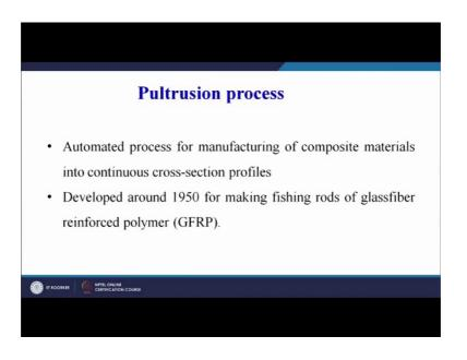
So, pultrusion process, it is automated process, we will also try to understand it with the help of a diagram as well as a simulation or the animation. So, automated process for manufacturing of composite materials into continuous cross section profile.
