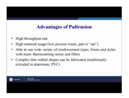
So, it is can be use our mass production, high throughput rate, high material usage, low process waste part is net. So, I think in the last or last to last session I have a tried to explain a near net part. So, near net part means, the final product is exactly the product which we have designed, and that we are going to use that it may not require any further processing. So, near net part is being produced
