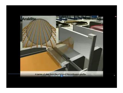
After being wet, a series of die forms the shape of the pultrusion profile. So, this series of dies can be called as the pre former as per our schematic diagram. So, these pre formers will give shape to the fibres, which are already impregnated with the resin.
