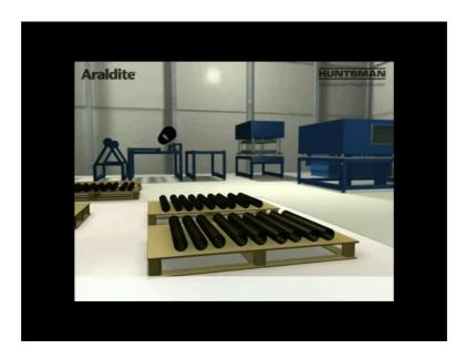
So, it is cutting the profile, and these are the final profiles, hollow profiles, or hollow cylindrical profiles made by the pultrusion process.
