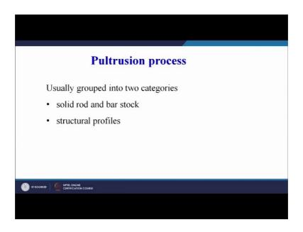
It is usually grouped into two categories; solid rod and bar stock as well as structural profiles. Now what are the raw materials that are basically used for pultrusion process. The reinforcement can be glass fibre, which can be e glass or s glass then.
