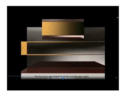
This is the movement, movement of the pultruded profile. Finally, the pultruded profile is coming out from here..
