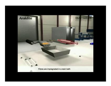
This is the fiber creel; the fibers are coming from the fiber creel. These are the fibers that are coming; this is called the pre former. The fibers are coming from here, they are going towards the resin bath, this is the resin bath continuous movement of the fiber, and they are here getting impregnated in the resin bath.
