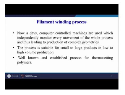
Now, nowadays computer controlled machines are used which independently monitor every movement of the whole process, thus leading to production of complex geometries. So, now, there are number of movements involved in the filament winding process.
