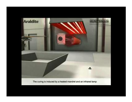
And finally, we will take this mandrel, hot mandrel for curing process. The curing is induced by a heated mandrel and an infrared lamp. So, the mandrel is also hot, and infrared lamp is used to further perform the curing operation. Now curing as all of, you know is the polymerization process, specifically in case of thermosetting type of resins. The curing is induced by a heated mandrel as well as the lamp. Now ones the tube is gelled, the mandrel is placed in oven for curing.
