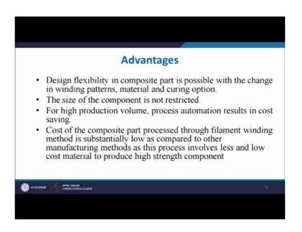
Design flexibility in composite part is possible with the change in winding patterns, material and curing options. So, that can lead to tailor made parts design flexibility is possible. The size of the composite is not restricted, we can have a long mandrel also, we can have a large carriage also. So, the model can be scaled up, and we can have a large size composite part, which can be made by the filament winding process.
