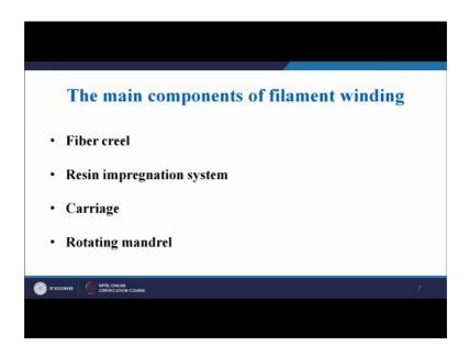
Then finally, the rotating mandrel is the final component which takes the fiber or wounds winds the fiber; that is impregnated in the resin bath, and that is coming from the fiber creel.
