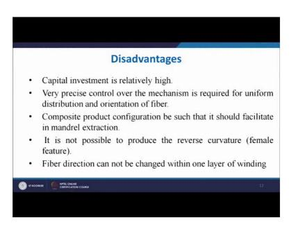
So, the capital investment as a cost of the machine is relatively high. Very precise control over the mechanism is required for uniform distribution orientation of fiber. So, the control is the key. If you control it precisely, you get a very good product. If you are not able to control it precisely, you may get a poor quality product, which can turn into a disadvantage also. Composite product configuration be such, that it should facilitate easy mandrel extraction.
