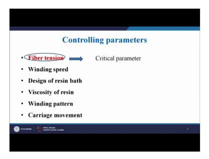
Now, what are the important controlling parameters. First one is the fiber tension, winding speed, design of the resin bath, viscosity of the resin winding pattern, carriage
