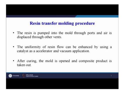
The mold is properly closed and clamped. The resin is pumped into the mold through ports and air is displaced through the other vents.
