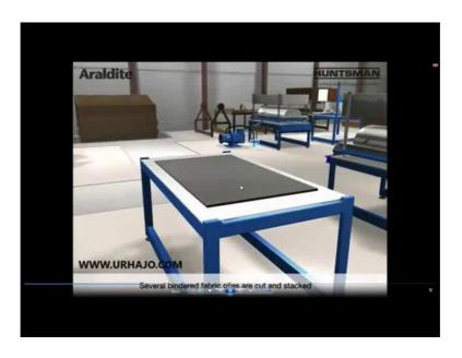
We will cut it as per the desired sizes. Several bindered fabric plies are cut and stacked together. Depending upon thickness of the final product required we will select these layers.
