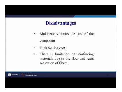
Now, mold cavity limits the size of the composite, high tooling cost. So, the tooling cost is high we have seen the steps involved in the complete process. And therefore, the tooling cost is slightly higher.
