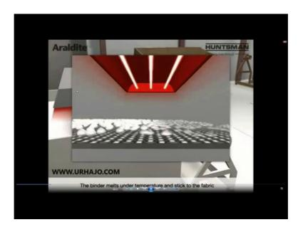
Then we are supplying the heat this is the heating arrangement, and this is the layer of fiber that is moving and this is the binder being heated.
