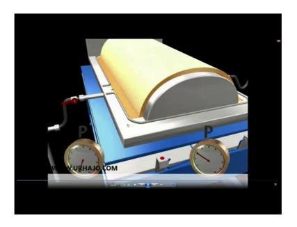
It will impregnate the fibrous preform that we have already introduced inside mold cavity; you see here the vacuum is stopped, when the resin exits the mold.
