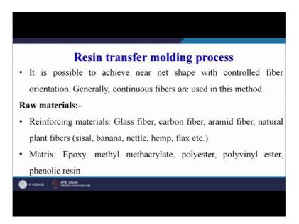
So, in resin transfer molding process it is possible to achieve the near net shape with controlled fiber orientation. Now 2 terms have come here in the sentence. The first one is near net shape. So, what we want is we will see in the animation? We will directly get our final product near net means near net. So, net means; the exact, but near net means
