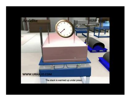
And now this is our fibers reinforcement. The stack is warmed up under press. So, we want to give it a desired shape. As we have seen this process can be used for making near net shape products. So, here the stack is warmed up under press, and we have given a definite shape to this fibrous form. This is fibers, may be 4 layers or 6 layers or 8 layers. It has now come out.
