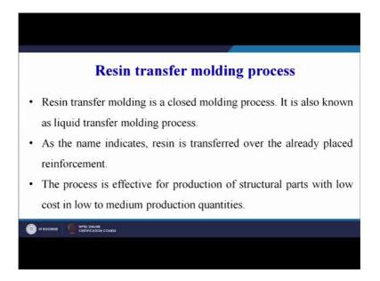
So, let us start our discussion now. The resin transfer molding process is a closed molding process. It is also known as liquid transfer molding process. So, we will be transferring our resin into the mold cavity, where we will have preplaced fibers already existing there. So, those fibers are already preplaced their they are already available there. Only thing is we have to supply the resin or the polymer, and the polymer and fibers then will combine together to make a composite product.
