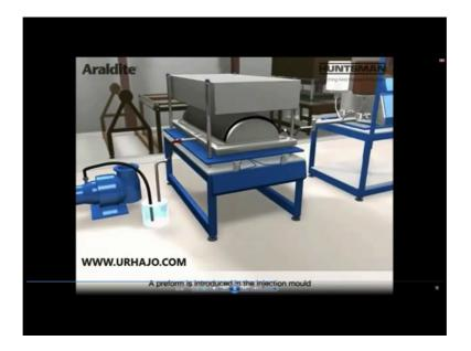
A preform is introduced in the mold. The vacuum pump removes the air and trapped. So, this is a vacuum pump it is trying to remove the air and trapped air, the resin is injected now.
