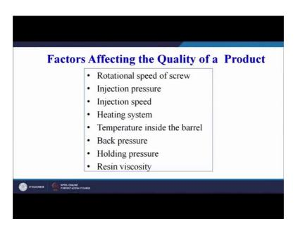
So, these are the factors that affect the quality of the product very quickly we can read these rotation speed of the screw, injection pressure, injection speed, heating system, temperature inside the barrel, back pressure, holding pressure, resin viscosity, and this list is not complete there can be other parameters also which can affect the quality of the product made by the injection molding process.
