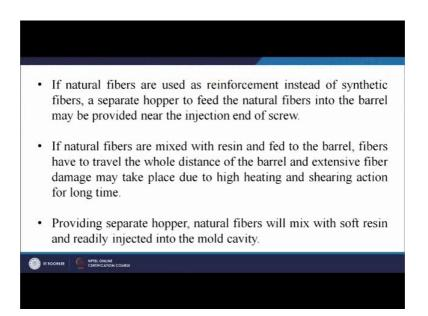
If natural fibers are used as reinforcement instead of synthetic fibers a special case because we know that in case of composites we can have synthetic fiber reinforcement, we can have a natural fiber reinforcement; a separate hopper to feed the natural fibers into the barrel may be provided near the injection end of the screw.
