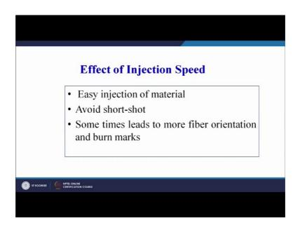
Now, what is the effect of the injection speed easy injection of material it will avoid the short shot that is the product may not be formed as per the dimensions sometimes leads to more fiber orientation and burn marks.
