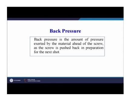
So, Back Pressure is the amount of pressure exhorted by the material ahead of the screw as the screw is pushed back in preparation for the next short of the next cycle.
