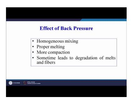
Then what is effect of back pressure it will lead to homogeneous mixing, proper melting of the raw material that is the polymer, more compaction and sometimes may lead to degradation of the melts and the fiber. So, we have to optimally select the back pressure. So, that no degradation of the fiber takes place.
