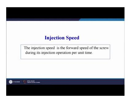
Injection speed is the forward speed of the screw during it is injection operation per unit time.
