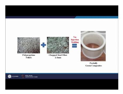
Here we have a Poly propylene pellet us this is a pellet form which is shown here, then we have chopped sisal fibers, this is one type of a natural fiber, the length of the fiber may range from 2 to 3 millimeter and this is a partially green composites this will be exact, we can say product that we want to make which is a partially green composite because polypropylene is a non biodegradable polymer, but the fiber that we are using is a natural fiber.
