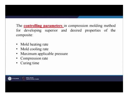
The controlling parameters in compression molding method for developing superior and desired properties of the composite product are, as I have already told you mold heating rate, mold cooling rate, maximum applicable pressure, compression rate, curing time.
