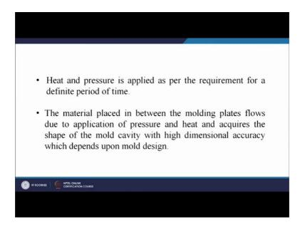
Heat and pressure is applied as I have already highlighted as per the requirement for a defined period of time, third thing that I have missed was the period of time, there has to be a time domain also. So, we have 2 important things here one is the pressure, another one is the heat and the third part is the time holding time usually we call it that for how long the material is there inside the mold cavity.
