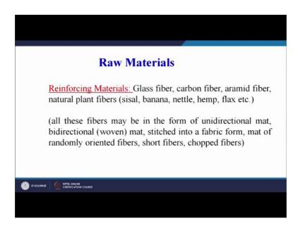
The first one is a reinforcing material that is glass fiber, carbon fiber, aramid fiber, natural plant fibers can be there like sisal, banana, nettle, hemp, flax etcetera, all these fibers may be in the form of unidirectional mat, bidirectional, stitched into a fabric form, mat of a randomly oriented fiber, short fibers, chopped fibers. If you remember in the last 2 processes we have seen in case of hand layup process majorly we will use even mat
