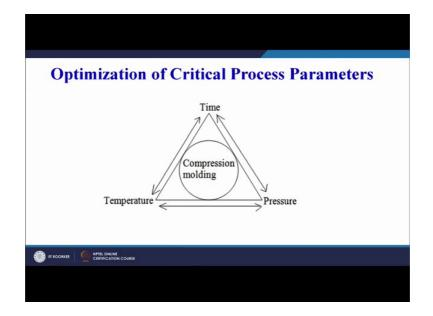
But 3 major parameters that are important are the time, the pressure and the temperature, we have to supply heat, therefore, temperature is important we have to cool it, time is important and we have to apply the pressure, we have consolidate our composite product therefore, the pressure is very very important.
