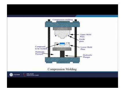
This is the upper mold plate this part and you can see this shape that I am emphasizing is the exact duplicate of this shape. We can see what type of product we will get this is the compound to be molded it as I have told you specifically in case of thermosetting type of polymer.
