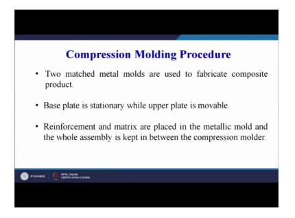
So, two matched metal molds are used to fabricate the composite product, the major point here to address is the shape of the mold, size we have already seen small to medium, the mold will not be a very large size, mold will be of small to medium size, but the shape is important the shape of the mold should confirm to should be the exact replica or the duplicate of the final product that we want to make.
