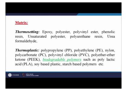
Thermosetting can be a epoxy, polyester, polyvinyl ester, similar to what we have already seen in hand layup process and spray layup process. Similarly in thermoplastic we can use polypropylene, polyethylene and sometimes we can also go for biodegradable polymers such as poly lactic acid, soy based plastic or starch based polymers. So, we can use both we can use thermosetting type of polymers also we can use thermoplastic type of polymers also.
