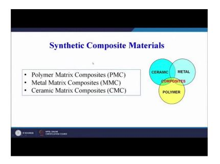
This classification is a most commonly adopted classification for composite materials. Now in this classification; you can see that we can classify the composite materials based on the matrix that is used for making the composite. And here you can see; as the name suggests; polymer matrix composite, metal matrix composites, ceramic matrix composites. So, you should remember that based on the 2 constituents; you have a classification.
