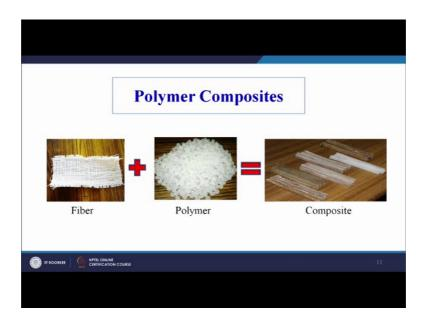
And once we have the natural fibers, we have the polymers which are the readily available; we can make a composite material. On your screen you can see, the fiber when
