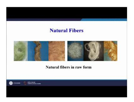
On your screen this is a list showing different types of natural fibers, they are in the raw form; they can be woven into the mat form and then the mat can be used as a reinforcement for making natural fiber reinforce laminated composites. But this is just showing the raw type of fiber which are available and these are these have been derived from nature.
