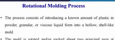
• The mold is rotated and/or rocked about two principal axes at relatively low speeds as it is heated so that the plastic enclosed in the mold adheres to, and forms a layer against, the mold surface.
