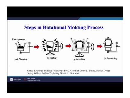
A diagram is very you can say well representing the whole process that we have already understood. You can see here this is the mold, split mold this is one half of the mold the top half of the mold will close this mold and then the rotation has to be done.
