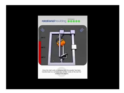
And on the screen you can see the maximum temperature attainable is 270 degree. So, the rotation now along the axis.
