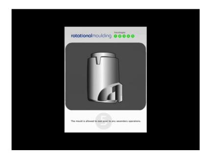
So, once it has cooled the mold opens and finally, the product comes out of the mold that is the ejection step. So, 4 major steps are there that is charging heating cooling and part ejection. Now I think we have already discussed and I have explained the process parameters that we can control.
