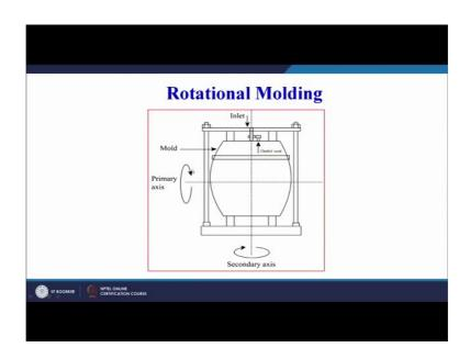
This is the primary axis dotted line is shown here primary axis and then there is a secondary axis this line is the secondary axis.
