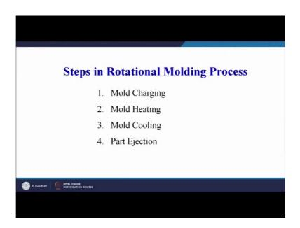
First is the mold charging. Mold charging means adding the raw material in the form of granules in the form of powder in the form of viscous liquid into the rational mold or into the mold. So, that is called mold charging. Then mold heating means heating the mold. So, that the charge that we have added into the hollow mold melts and attain sufficient viscosity.
