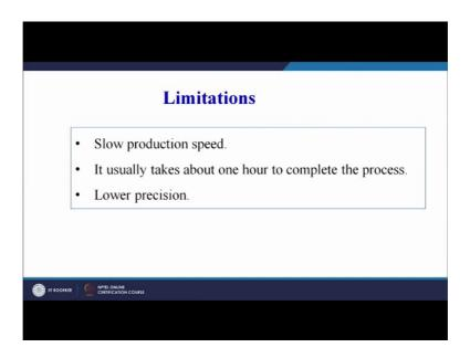
It usually takes about one hour to complete the process that depends upon the shape the complexity of the final product, but in generally it may take a cycle time of 30 minutes to one hour and the precision is slightly less as compared to the injection molded products.
