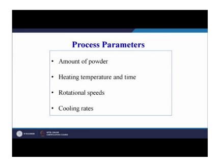
So, first is the amount of powder or charge it can be granules also it can be viscous liquid first thing is amount of raw material that we are adding into the hollow mold. Heating temperature and time.
