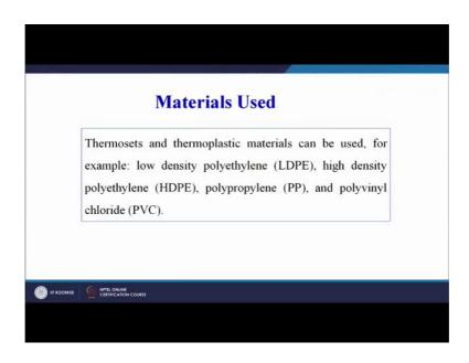
For example, low density polyethylene LDPE HDPE polypropylene and polyvinyl chloride that is PVC. So, LDPE HDPE PVC PP all these polymers can be used as raw materials for making products using the rotational molding process.
