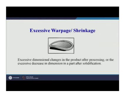
So, the first part is warpage; that is excessive dimensional changes in the product after processing; that is warpage and shrinkage is the excessive decrease in the dimension of the part after solidification. So, we are addressing both together the warpage and the shrinkage.
