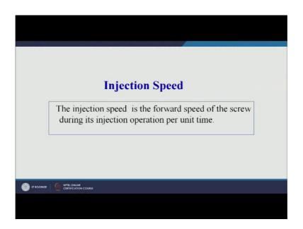
Now, injection speed is the forward speed of the screw during it is injection operation. So, the screw will be rotating. Then it will be moving forward to push the material into the mould cavity. Not during that movement whatever what is a distance it travels per unit time that is called the injection speed.
