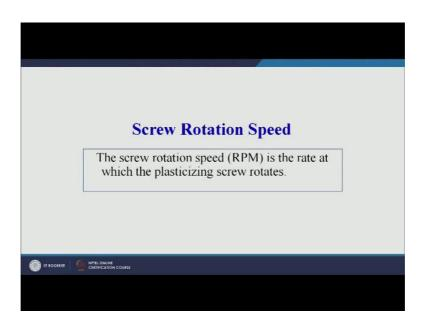
So, screw rotation speed that is RPM is the rate at which the plasticizing screw rotates. So, that is the rotational speed of the screw, and that also needs to be optimized. Now what are the purposes or the objectives of the screw. As all of us know it is feeding it is mixing, it is melting, it is metering.
