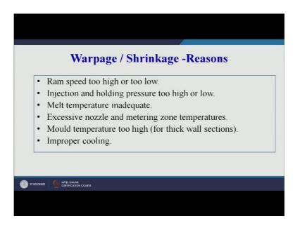
Now, what can be the reasons for warpage and shrinkage? Ram speed too high or too low ram speed, we can say if we are using a plunger type of arrangement for pushing the molten plastic into the mould cavity. So, that is speed if it is too high, it can lead to warpage and shrinkage and if it is too low the again we can get warpage and shrinkage. Therefore, it is important to judiciously select the ram speed. Injection and holding pressures too high or low.
