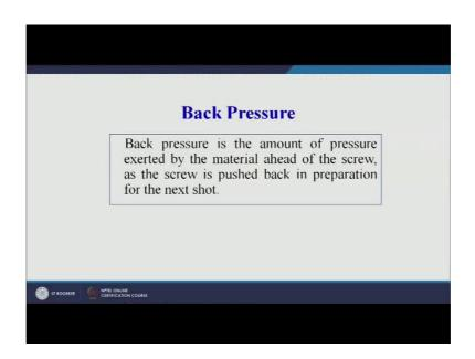
Now, what is back pressure back? Pressure is the amount of pressure exerted by the material ahead of the screw. Now then the screw will rotate it will certainly have some material in front of the screw after you have injected this back pressure will apply pressure or a force on the screw and a screw will be pushed back.
