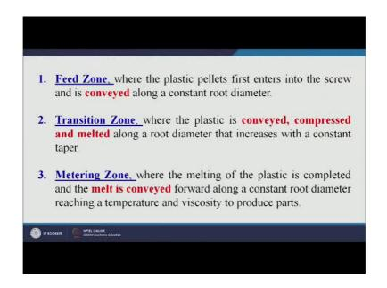
Now, just I have tried to explain what each section of screw will do, but let us read first for better understanding. Now feed zone; where the plastic pellets as I have told plastic pellets or granules, first enters into the screw and is conveyed along the constant root diameter. So, the feed zone is the zone where the screw will receive the pellets from the hopper.
