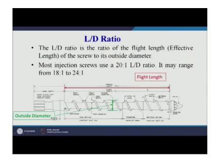
So, means that the length as is specified in the diameter, sorry in the figure also you can see the length is 20 times that of the diameter.
