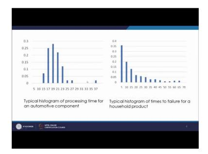
So, we see here that this is the typical histogram for processing time of in automotive component and this is the histogram of time to failure for a household product, it looks like as if it is exponentially distributed if you look at.
