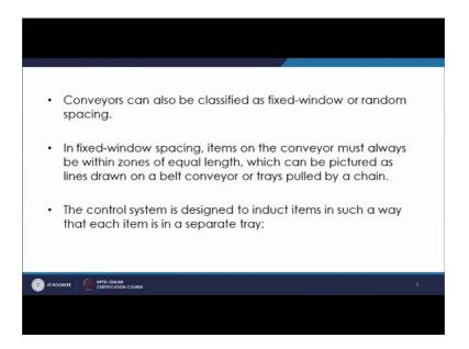
Conveyors can also be classified as fixed window or random spacing. So, either it is fixed window or it is random spacing. So, what happens in the fixed window spacing that items on the conveyor must always be within zones of equal length? So, that is known as fixed window type of spacing for the conveyors. So, which can be so, you have the lines
