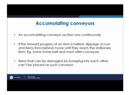
Now, in the case of accumulating conveyors it is said that they run continuously. So, the conveyor section will run continuously and if the forward progress of an item is halted then there will be sleepers occurring. So, what will happen? The item from behind; it will move until they reach the stationary item. So, there are 2 items and that will be stopped.
