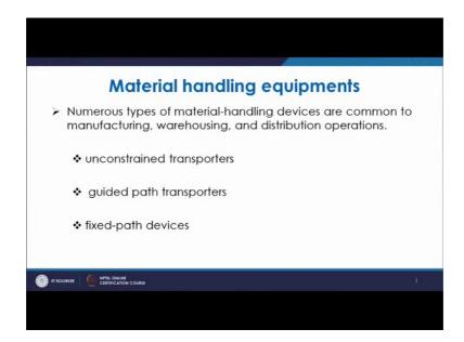
Now, what are the normally material handling equipments which are used in the manufacturing industries? So, you have the common equipments which are used in this manufacturing or warehousing or distribution operations are basically categorised in you know normally they are categorised as accumulating as well as non accumulating then that basically comes under this unconstrained transporters. So, we have the first one is unconstrained transporters.
