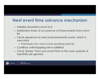
So, in the next event time advance mechanism, we are initialising the simulation clock to 0. As it is written that you initialize this simulation clock to 0. So, when you are starting the simulation, certainly you are normally starting at a 0 time. So, initially it will be at 0 time.
