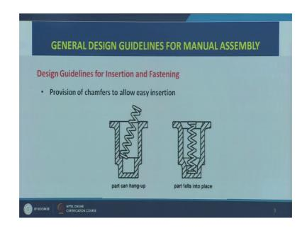
So, that the product is assembled easily; this is another example you can see design guidelines for insertion and fastening again as we have discussed there are 2 broad categorization of the manual assembly operations the handling and the insertion and fastening. Now we are looking at design guidelines for insertion and fastening and this is another guideline for insertion and fastening.
