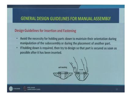
Now, here we can see design guideline again for insertion and fastening avoid the necessity for holding parts down to maintain their orientation. Sometimes we need to design the part in such a way that it is self oriented here we can see there is no position. So, this will move here and there and we have to insert ensure a certain that this particular hole or this particular feature matches with the feature in the basic or the base part or the part to which this part has to be assembled.
