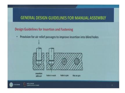
So, this is the design guidelines for insertion and fastening; this is another guideline this is here we can see this is a blind hole insertion is difficult this is the part which is going inside this blind hole. So, we should what we should do we should provide for air relief passages to improve the insertion into blind holds.
