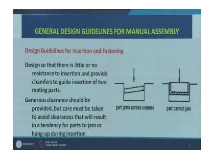
Now, first part we have seen that there are 2 parts in manual assembly; first part is the handling part, another part is the mating part or the insertion or fastening or the actual operation that is done. So, when we are designing a product we should see that we design the part in such a way or design the component in such a way that it is easy to assemble by insertion and fastening.
