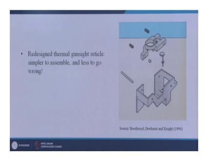
As per this guidelines if you redesign this part it you can see how simpler same objective met, same functionality, no compromise in the performance simpler part. So, redesign thermal gun sight reticle similar to simpler to assemble and less to go wrong.
