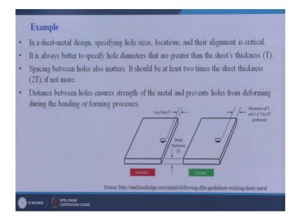
It is the sheet metal product you can see. In a sheet metal design specifying the hole sizes locations and their alignment is very very critical. So, you can see hole sizes in critical, location of the hole is also very critical because here we are this example is related to the location of the hole in the sheet metal. So, it is always better to specify hole diameters that are greater than the sheets thickness. So, this is a sheet which has got a thickness of T capital T.
