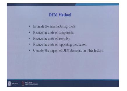
Now for the DFM I said just a brief summary estimate the manufacturing cost, reduce the cost of the component without compromising the performance. Reduce the cost of assembly without compromising the reliability durability. Reduce the cost of the supporting production whatever we are saying indirect cost and consider the impact of DFM decisions on the other factors as well.
