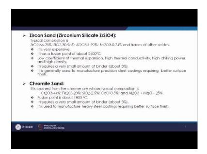
Very expensive it is expensive, but it has high refractoriness values. It has refractoriness value of degree 2400 degree centigrade. It has other qualities like low coefficient of thermal expansion high thermal conductivity high chilling power and high density. So, if you take in the advantage mode these high chilling power high thermal conductivity they will certainly increase the grain properties or the fineness of the grains near the boundaries of the of the casting.
