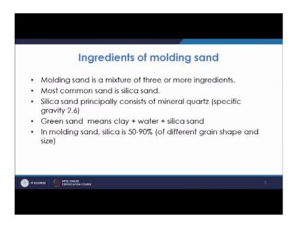
Now, what is the ingredient of molding sand? In molding sand basically you have 3 or more ingredients. So, in that you have normally clay plus water plus silica sand. If you take the silica sand as the normal molding because mostly the silica sand is used as the molding sand, in that case you have silica sand plus clay plus water, but then apart from that you also use adhesives that we will discuss later.
