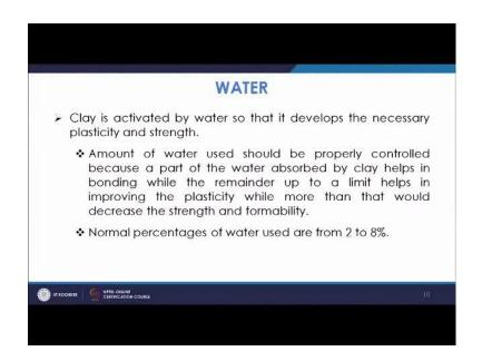
Then the use of water because waters purpose sees purpose of water is to activate the clay and form a bond between the clay because clay is being coated on the sand and the water quantity has to be maintained. So, that the optimum strength of the molding sand is achieved. So, you have tempered water and water percentage is normally from 2 to 8 percent. So, this is how you get a good mold having good molding properties, good properties what we require.
