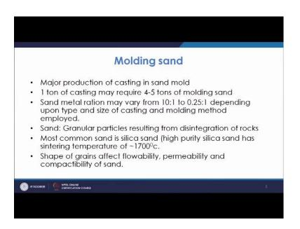
Sand metal ratio may vary from 10 is to 1.25 is to 1. So, depending upon which type of process you are using that is type and size of casting and molding method is employed you may have the sand metal ratio. So, if you are having a metal casting of suppose 10 kg, sand may vary from 100 kg to maybe 2.5 kg. So, basically it depends which kind of molding method you are using which kind of sand you are using with binders and what is the type and size of the casting.
