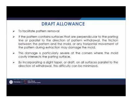
So, that may damage the mold, even at the corners it is more severe. So, you need to be careful in providing certain allowance, that it can you can take it without damaging the mold. So, you give a slight taper may be one degree to two degree. So, that it can take and that depends upon the dimension of the vertical surface.
