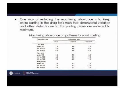
This is one of the ways that you do the casting in the drag part itself, there are certain data given for machining allowance you can see depending upon the dimension you have certain part in the cope and surface and the bore portion. So, this is normally used for centerizing the allowanced values in machining.
