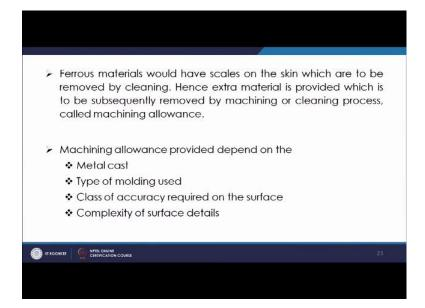
So, machining allowance depends upon metal cast, which is which metal you are casting, type of molding used, class of accuracy and complexity that we have already discussed. What kind of material you are using? What kind of accuracy we want? All these things are required. One way of reducing the machining allowance is to keep entire casting in drag flask that dimensional variation of and other defects due to parting plane are reduced.
