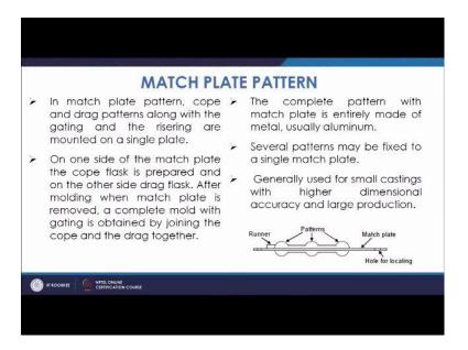
So, the only difference between the match plate pattern, and the cope and drag pattern is that in the cope and drag pattern you use separate pattern plate, match plate, where you one plate is used for making the cope pattern another is used for drag pattern in the case of match plate pattern, you have the same match plate which is or plate which is used for making the pattern for both the halves cope as well as drag.
