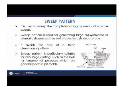
It is basically used for axi-symmetric shapes, and once you have the sweep of certain shape and if you rotate it along a vertical axis, on all the directions you will have a cavity bed of this shape on all the sides and in that basically you can do the casting.
