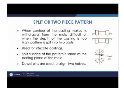
So, they that are pins are dowel pins, they are used so that, there is proper alignment between the two parts and these are known as a split or two piece patterns and this surface split surface will be taken as the parting plane of the mold.
