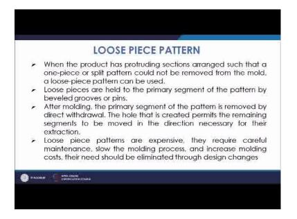
Next type of pattern is, loose piece pattern. So, basically many a times you have the cavity, to be made in such a manner that are certain portion if you make the pattern in a unified way it is difficult to take the pattern out in those cases, you are providing very loose piece of the pattern material at that place which can taken out separately so, that the whole pattern from the cope or the drag portion can be taken out separately.
