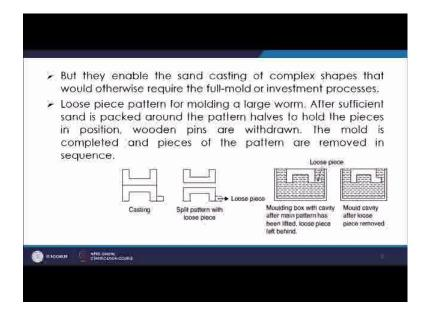
They enable the sand casting of complex shapes that would otherwise require the full mold or invest. So, otherwise you will have to go for very complicated or specialized type of casting process, and that will be costly.
