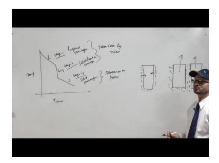
This is liquid, this is liquid plus solid and this is solid stage. Now, under this these stages there is decrease of temperature so, basically because of the decrease of temperature there is shrinkage.
